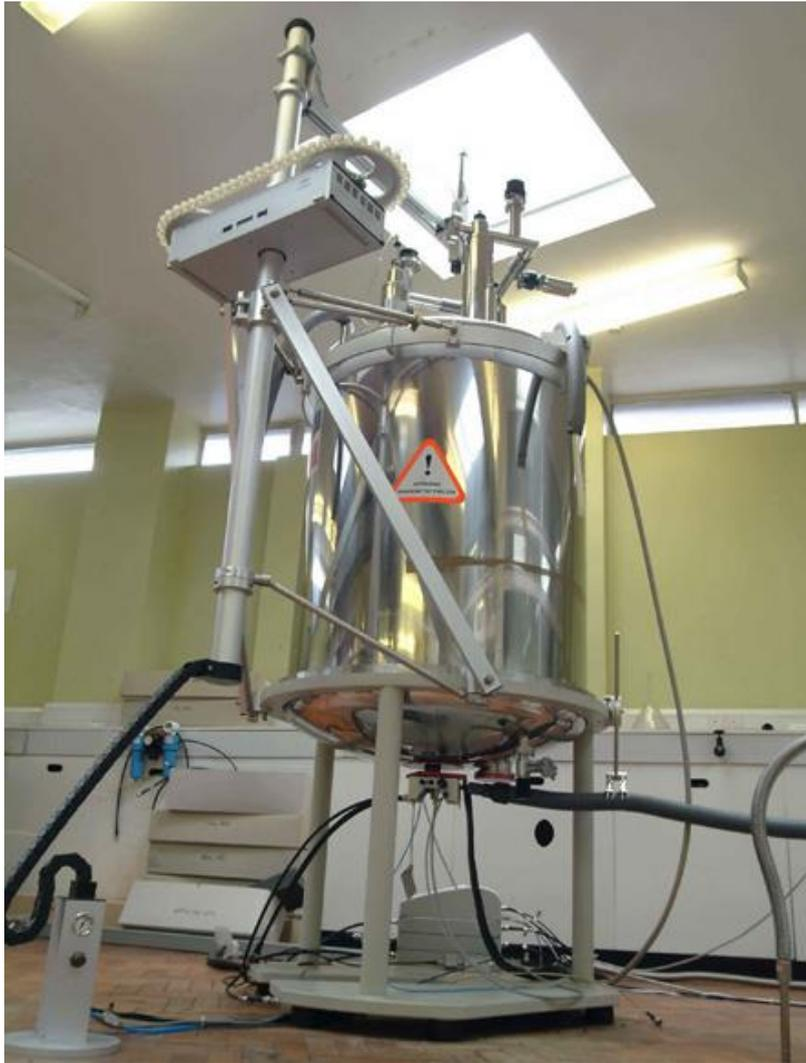
High frequency NMR spectrometers require very strong magnetic fields, which are produced using super-cooled coils ( $T = 4.2\text{K}$ , liquid He). The superconducting coils are surrounded by a giant vessel containing liquid  $\text{N}_2$ .
