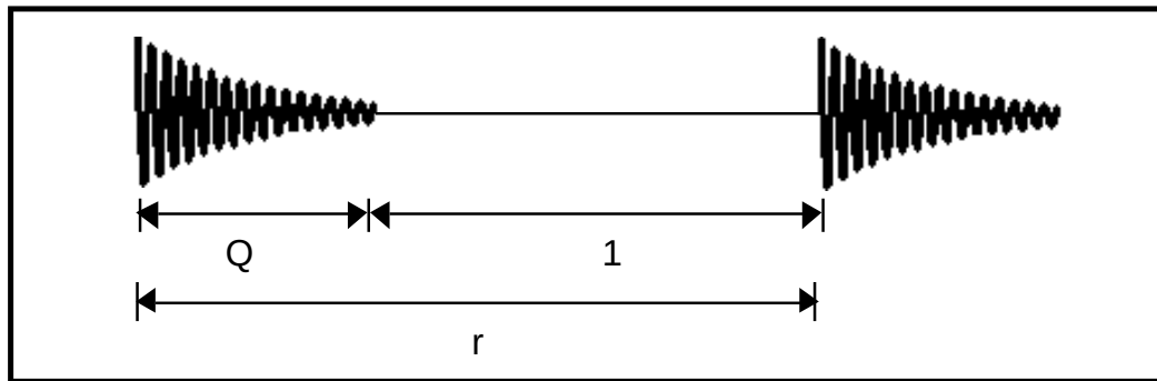
FIGURE 14. Definition of the recycle delay.
