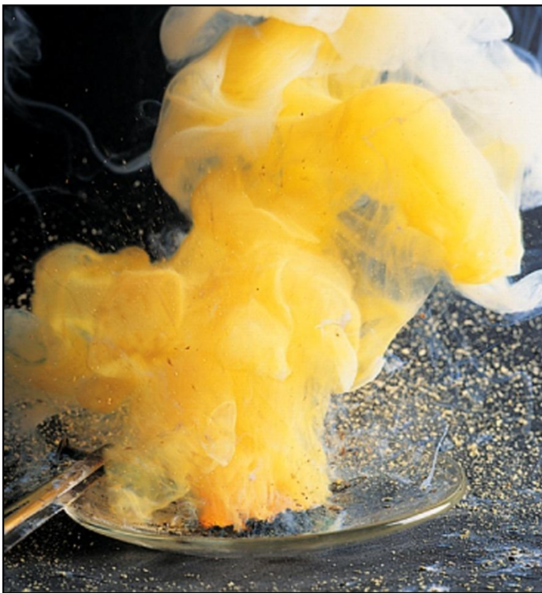
← Fig. 9.1 When a hot nail is stuck into a pile of zinc and sulfur, a fiery combination reaction occurs and zinc sulfide forms.
