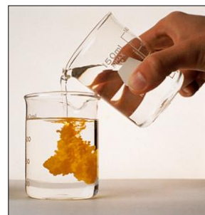
→ Fig. 9.2 A double-replacement reaction involving solutions of potassium and lead nitrate produces yellow, insoluble lead iodide as one of the products.
