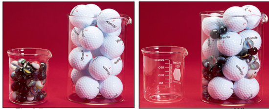
Fig. 8.7 When volumes of two different liquids are combined, the volumes are not additive.
