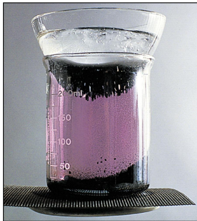
(b) Iodine has an appreciable vapor pressure even below its melting point.
