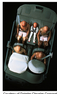
← Fig. 6.10 Testing apparatus for measuring the effects of air bag deployment.
