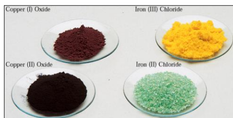
Fig. 4.7 Copper (II) oxide is black, whereas copper (I) oxide is reddish brown. Iron (II) chloride is green, whereas iron (III) chloride is bright yellow.
