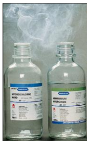
← Fig. 10.3 A white cloud of finely divided solid \text{NH}_4\text{Cl} is produced by the acid-base reaction that results when the colorless gases \text{HCl} and \text{NH}_3 mix.
