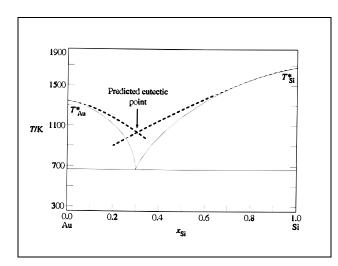
where, if we provide a composition  $x_{Au}$ , the equation predicts the temperature at which liquid with that composition is in equilibrium with pure Au(s). A similar equation can be written for Si using the enthalpy of fusion of Si and the melting point of pure Si to predict the curve ce on the right-hand-side of the equation. The intersection of these two curves will be the eutectic, e, if the assumptions made in Eq. (18) are valid over the entire
