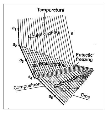
The variation of the length (of time) of the line segments (l,s), (l',s'), and (l'',s'') are related to the amount of solid that precipitates out of the liquid during cooling. Finally, when the composition of the system reaches the **eutectic point** (the minimum melting point composition), the system behaves like a pure substance. The figure to the left establishes this relationship.
