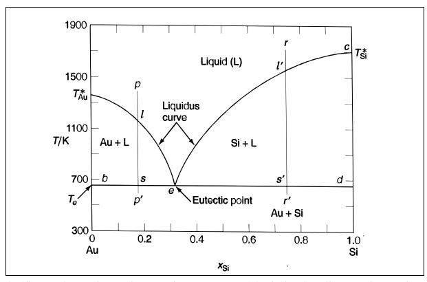
The figure above shows the Au-Si system. Eq. (6), derived earlier, can be used to predict the boundaries between the solid-liquid region [(Au + L) or (Si + L)] and the single phase region:
