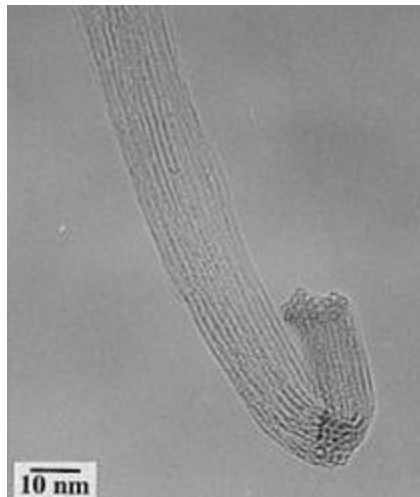
Figure 2-10: TEM images of a bundle of SWNTs catalysed by Ni/Y (2:0.5 at. %) mixture, produced with a continuous laser.
