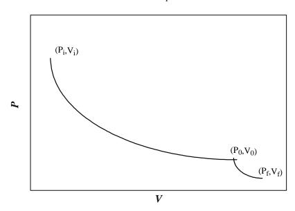
Isothermal expansion to  $(P_0,V_0)$  followed by adiabatic expansion to the final state:
